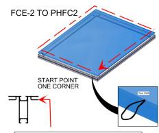
Install graphic by pressing the FCE-2 into the channels of PHFC2 extrusion. To pull graphics out of the channels, use tabs on the front side
