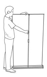
3. Release the lower lock and pull up the middle pole to adjust the height of the graphic.
