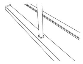
2. Release the upper lock and pull out the upper pole, then lock. Pull out the graphic and position the plastic end tip into the top profile.
