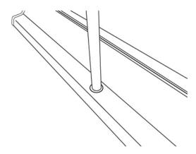
3. Pull up the graphic and position the plastic end tip of the pole into the profile.
