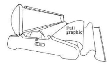
7. Push the graphic forward slightly to activate the spring system. Remove the locking pin and let the graphic retracts into the system slowly.
