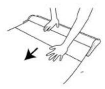
Stop the roller by inserting the pin into the hole on the right end plate completely.
