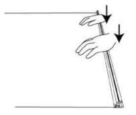
3. Open the cover by clicking at the two buttons at both ends and take out the internal roller.
