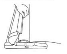
4. Slide the graphic out from the internal roller and the top profile, then follow the steps on "mounting graphic" instruction to install a new graphic.
