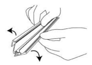
2. Insert the graphic into the profile and press hard.
