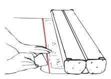
6. Remove the protective strip. Apply the graphic with picture side upwards and position along the red line.
