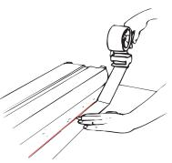
7. Apply packing tape over the joint!
