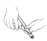
2. Use a flat blade screwdriver (or similar tool) to open the profile.
