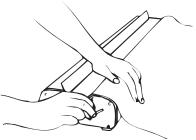
8. Grip the graphic and the base with your left hand. Remove the locking pin with your right hand. The mechanism is now activated!
