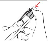
5. Press the plastic profile-lock into each end of the profile.
