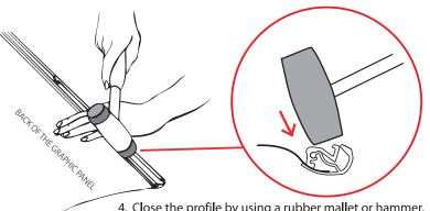
4. Close the profile by using a rubber mallet or hammer.
