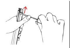
1. Use a flat blade screwdriver (or similar tool) to remove the plastic profile-lock from each end of the profile.
