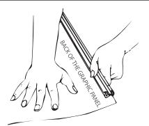
3. With the front of the graphic panel facing down, slide the profile onto the graphic.
