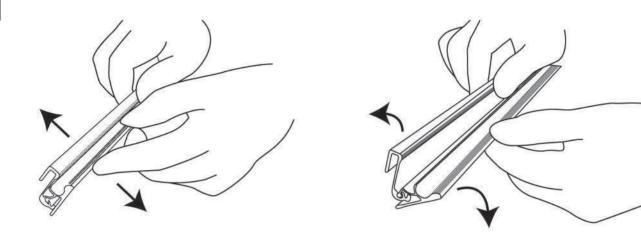
2. Insert the graphic into the profile and press hard.
