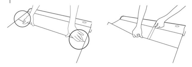
6. Press the graphic firmly and apply extra tape for reinforcement.
