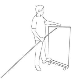
4. Insert the pole onto the cup of the base.
