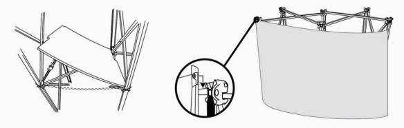
Place the tabletop on tops of the frame, and ensure the hubs went into the indents underneath the tabletop, so it will sit firmly.
