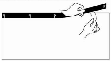
2. Follow the spacing distance from Mesa's line drawing, and mark the positions of mag tapes. Once marked, align mag tapes into its position and slowly remove the protection film at back of tape, to attach mag tapes to the graphic.
