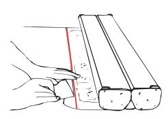
**3.** Remove the protective strip. Apply the graphic with picture side upwards and position along the red line.
