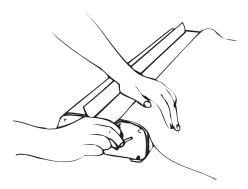
**6.** Grip the graphic and the base with your left hand. Remove the locking pin with your right hand. The mechanism is now activated!
