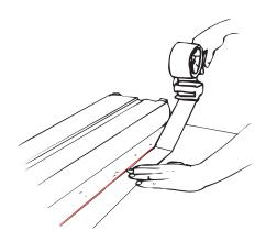
**5.** Apply packing tape over the joint!
