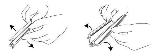
2. Insert the graphic into the profile and press hard.
