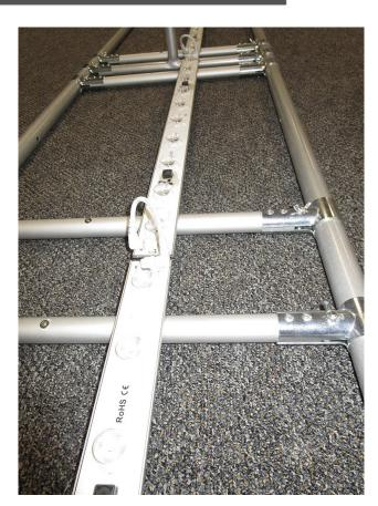
After tightening the white thumb screws as well as the wing nuts on the clamp bars to secure the lighting in place, use the short white cords to connect each LED light strip to one another, as shown in the image to the left. Repeat for the display's top light section.
