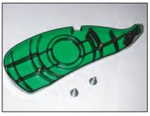
**Step 4**: Remove the plastic end cap to expose the pin that holds the tension on the display (indicated by the red arrow). **DO NOT REMOVE THE PIN AT THIS POINT**
