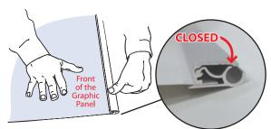
**Step 2**: Press down and secure the image in the snap profile. Start by pressing down on the outside and working in towards the middle.
