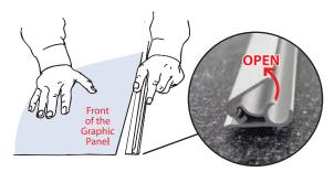
**Step 1**: Using a tool such as a flat blade screw driver, open the snap profile and insert the image.
