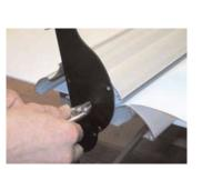
Rotate the flat bar clockwise. The table above indicates the number of rotations required for different size Banner Bug<sup>®</sup> models.
