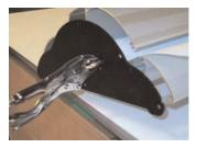
Position the left-hand end plate onto the system so that the flat metal bar of the reel protrudes from the slot in the end cap. Grip the flat bar with a vice grip.
