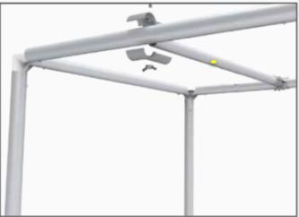
Without fully tightening the wing nut, install the clamp bars that house the LED light strips. Ensure the threaded holes (shown above in yellow) are facing toward the inside of the display. An even amount of clamp bars should be installed across the top AND bottom of the display. Note that there should be two clamp bars per one light strip.
